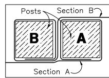
Figure 1: Top View of Roll-to-Roll Connection
