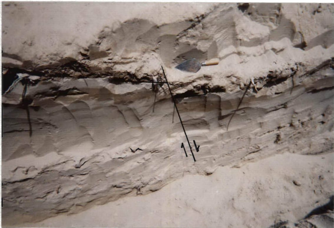
Photo 4. Bedding offset at trench Sta 0+23. Trowel on downthrown (east) side.
