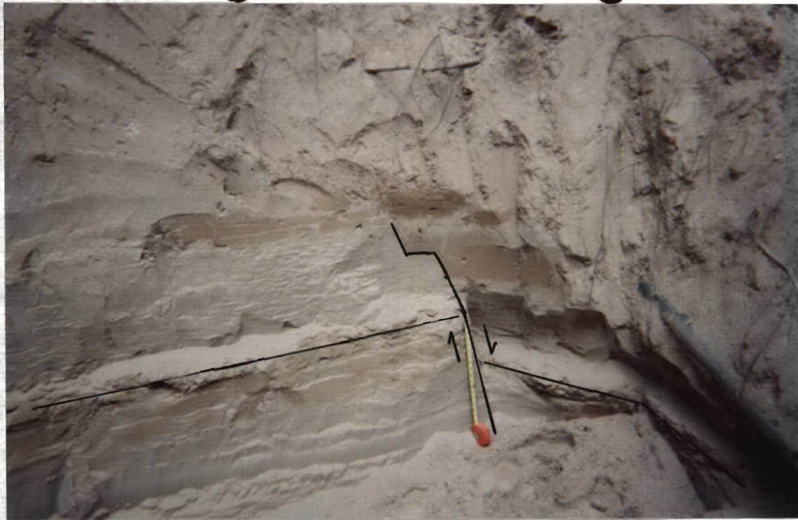
Photo 6. (Above) Stepped offset of bedding at Sta 0+57. Reservoir outlet and drain pipes at right of photo. Total vertical offset of lower clay layer is approximately 10 inches.
