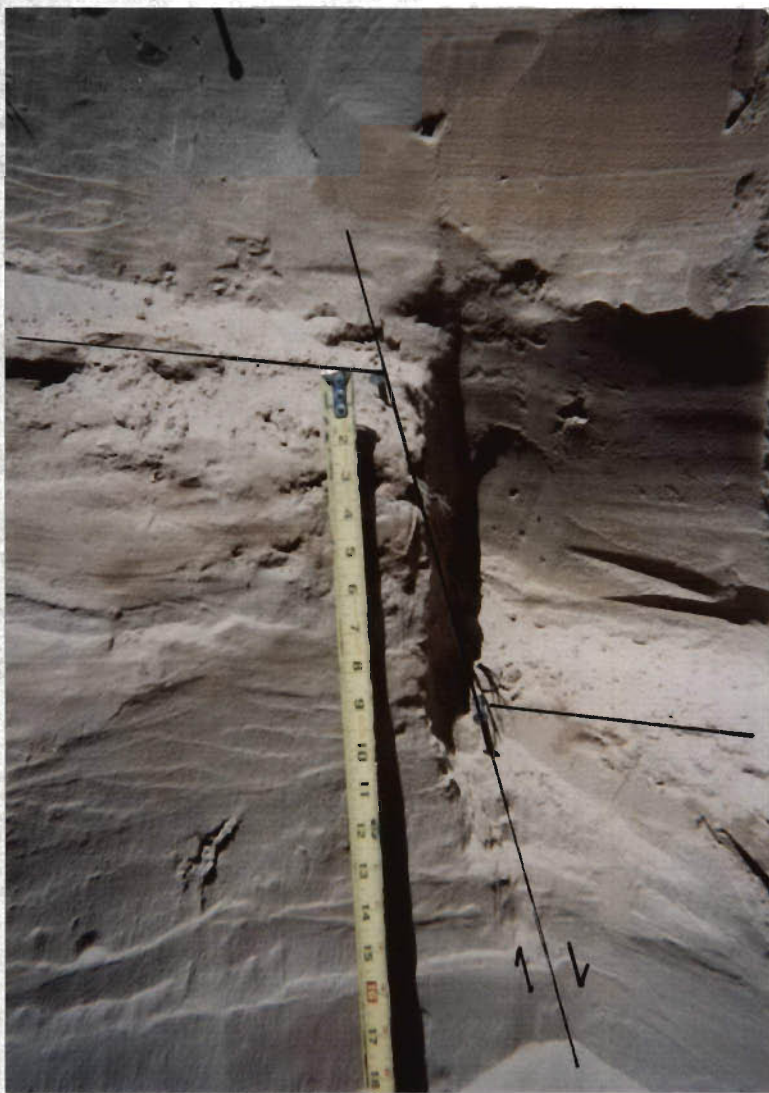
Photo 6. (Above) Stepped offset of bedding at Sta 0+57. Reservoir outlet and drain pipes at right of photo. Total vertical offset of lower clay layer is approximately 10 inches.
