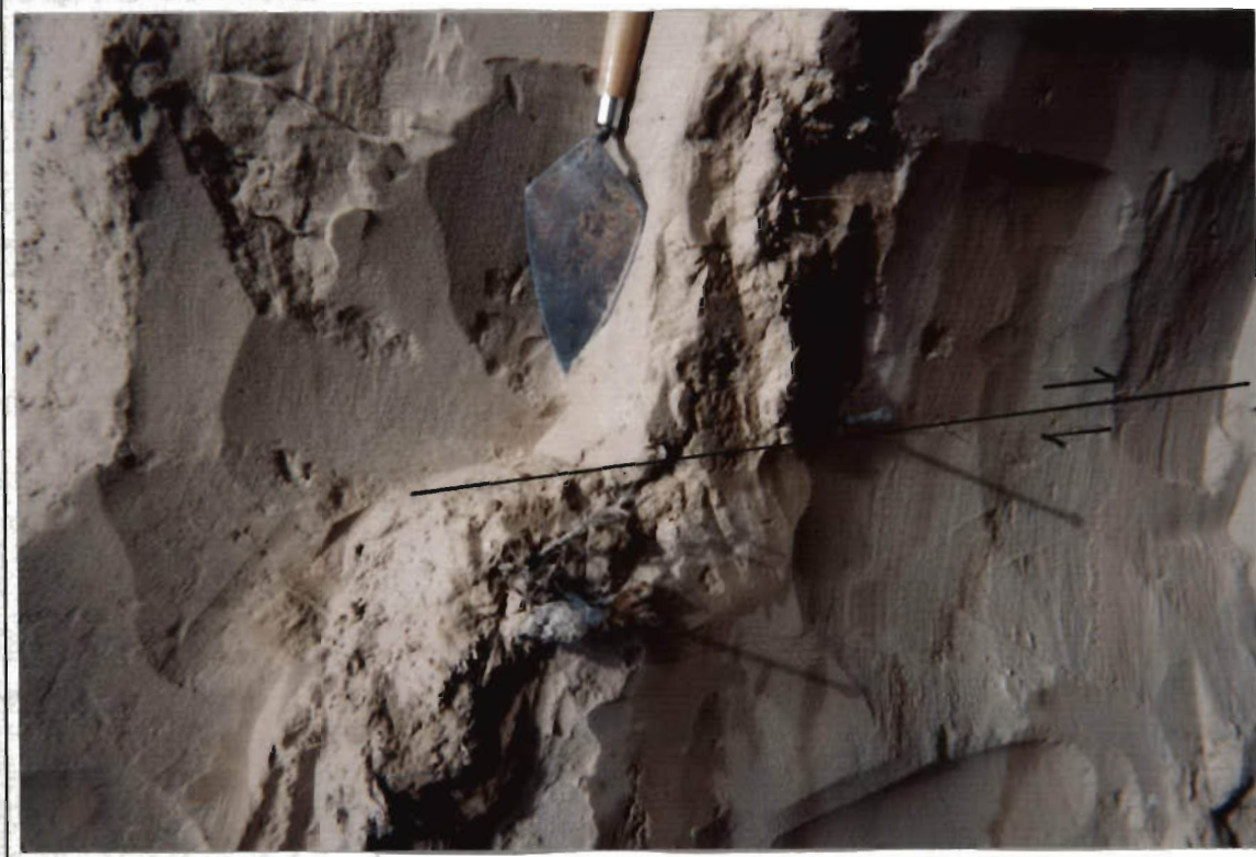
Photo 3. Close up view of offset bedding at Sta 0+23. Dark brown clay layer offset about 9 inches vertically. Trowel on downthrown side (east).
