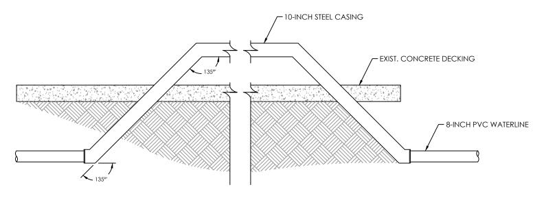
$\underset{\text{\tiny N.T.S.}}{\underline{\text{PIPE CROSSING DETAIL}}}$
