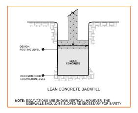
Over-excavation for structural fill placement below footings should be conducted as shown below. The over-excavation should be backfilled up to the footing base elevation, with Structural Fill placed, as recommended in the **Earthwork** section.
