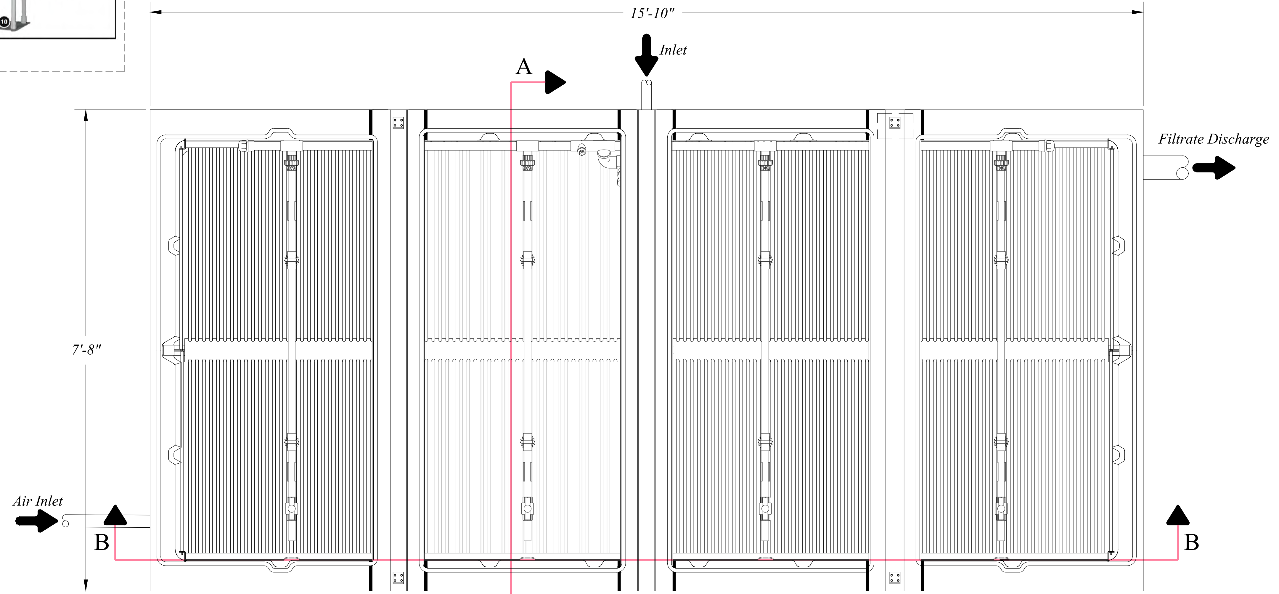
5 ORENCO FILTER POD ADVANTEX AX 100 DETAIL Scale: (NOT TO SCALE)
