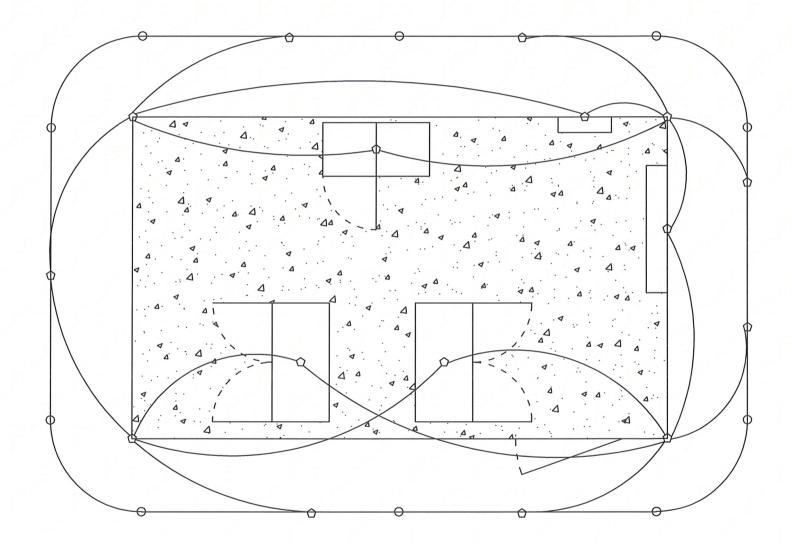
NOTE: TYPICAL GROUNDING PLAN SHOWN. CONTRACTOR TO TIE ANY NEW EQUIPMENT INTO EXISTING GROUNDING PLAN AT A MINIMUM OF TWO CONNECTIONS
