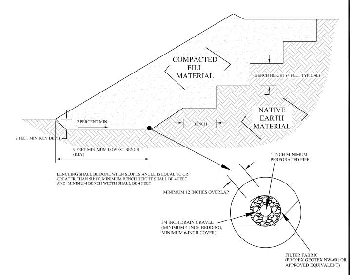
SUBDRAIN DETAIL (FOR FILL SLOPES IN EXCESS OF 15 FEET IN HEIGHT)
