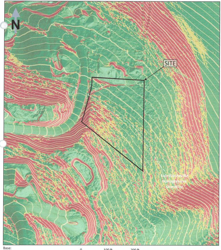
Base: 2016 LIDAR, 50cm resolution; slopes <25% shaded in green, 25-30% in yellow, and >30% red; 4-foot contour interval.
