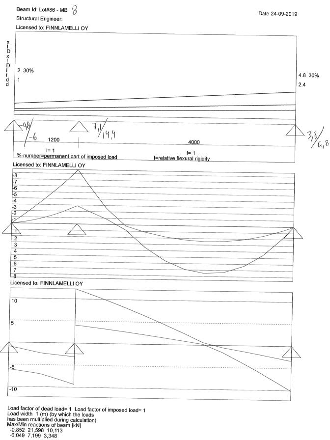
T24 164 x 260 B 2 Cf=1,00 Design method: Allowable stress design Increasing factor of the allowable stress 1,09 Factored Moment/Moment capacity [kNm] 8,602 19,351 44 % Factored shear force/shear capacity [kN] 12,241 29,770 41 %
