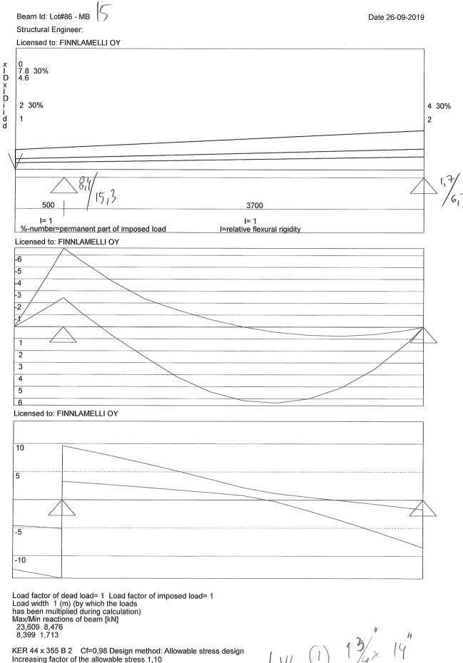
Increasing factor of the allowable stress 1,10 Factored Moment/Moment capacity [kNm] 6,589 17,884 37 % Factored shear force/shear capacity [kN] 13,989 19,391 72 % LUC (1) 13/x 14"
