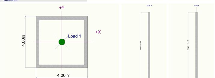
Sum infl M+S 0,89 (must be<=1) x= 3899 M=84,79 S=152,1 Deflection due to unfactored load (Deflection limit L/360)/L/180)! 0,0 mm (3 %) 8,0 mm (80 %) 0,3 mm (6 %) 4,1 mm (51 %) Attention! Ultimate limit design! Remember the load factors!!
