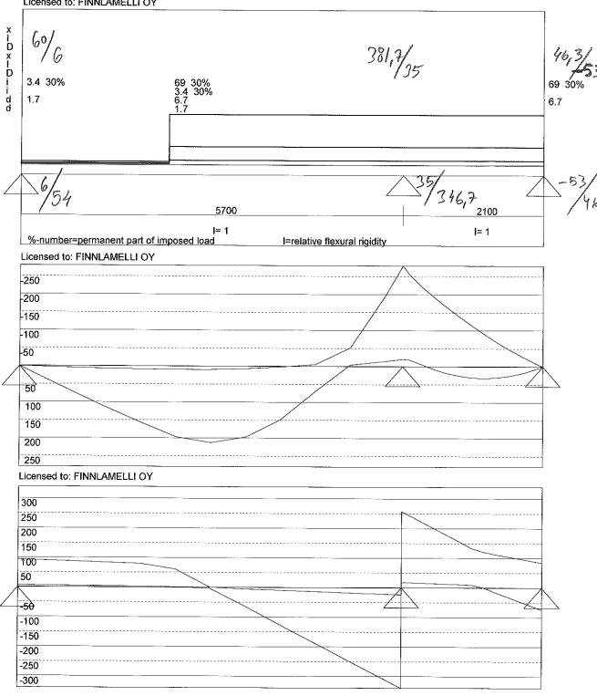
Load factor of dead load= 1.2 Load factor of imposed load= 1.6 Load width 1 (m) (by which the loads has been multiplied during calculation)
