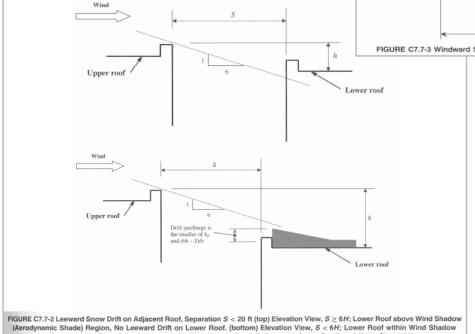
(Aerodynamic Shade) Region, Leeward Drift on Lower Roof; Drift Length Is the Smaller of (6H - S) and  $6H_D$
