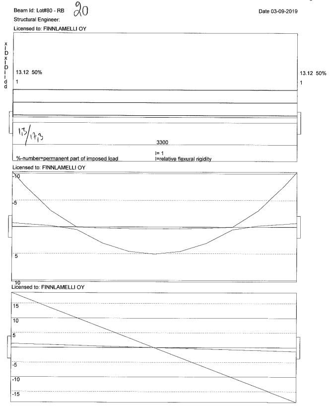
Load factor of dead load= 1 Load factor of imposed load= 1 Load width .8 (m) (by which the loads has been multiplied during calculation)
