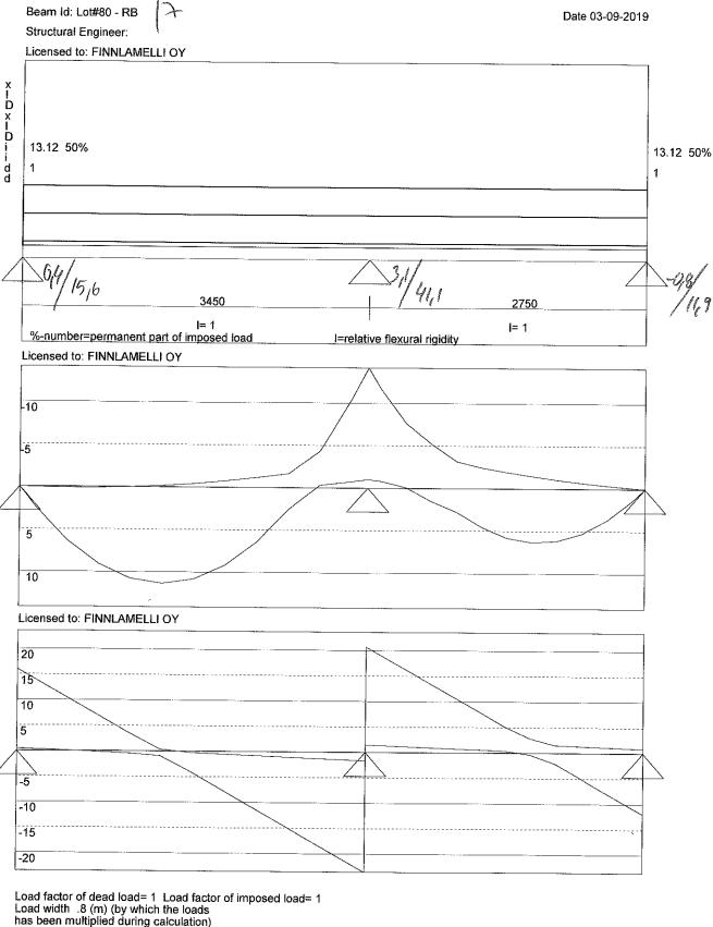
Load factor of dead load= 1 Load factor of imposed load= 1 Load width .8 (m) (by which the loads has been multiplied during calculation)
