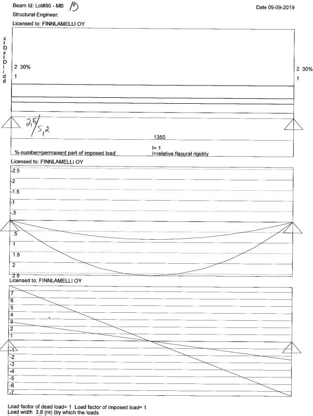
Load factor of dead load= 1 Load factor of imposed load= 1 Load width 3.8 (m) (by which the loads has been multiplied during calculation)
