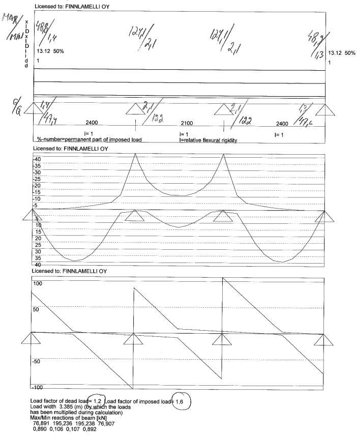
HEB 140 (Class of section=1/1) G= 33,7 I(cm4)=1509 W(cm3)=216 fy=235 Factored Moment/Moment capacity [kNm] 42,569 57,810 74 % Factored shear force/shear capacity [kN] 107,871 126,336 85 %
