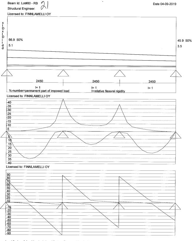
Load factor of dead load= 1 Load factor of imposed load= 1 Load width 1 (m) (by which the loads has been multiplied during calculation)
