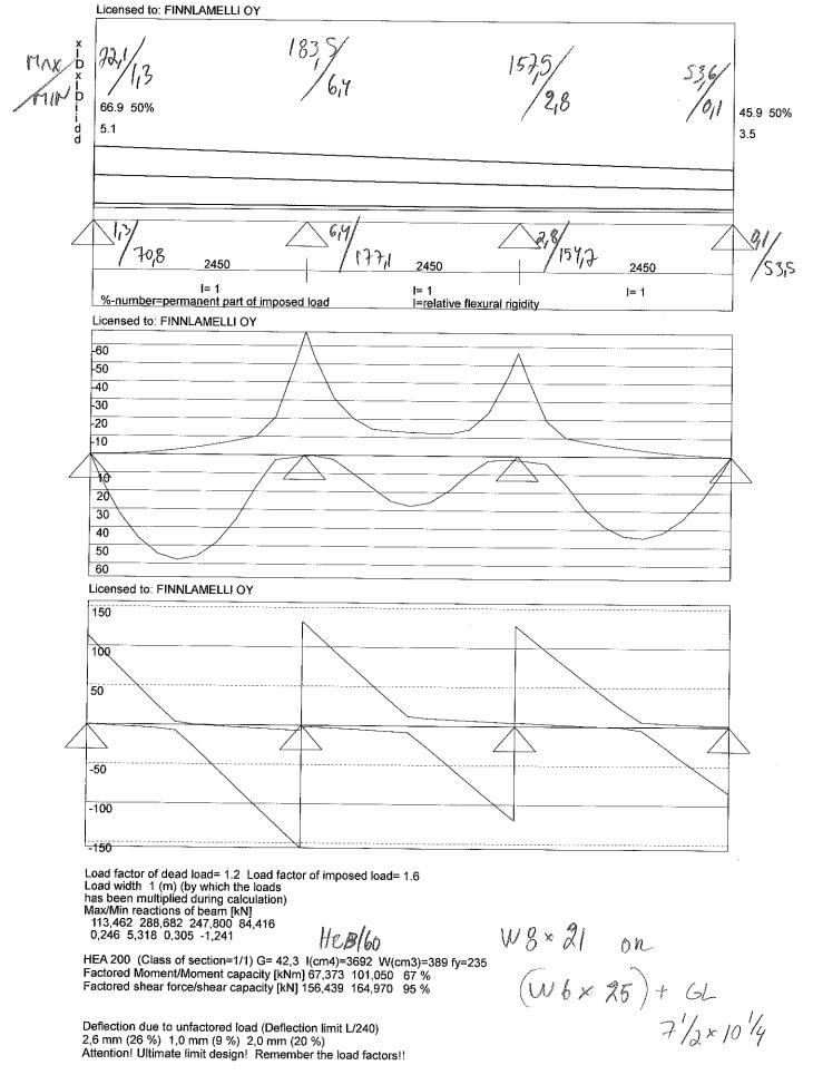
HEA 200 (Class of section=1/1) G= 42,3 I(cm4)=3692 W(cm3)=389 fy=235 Factored Moment/Moment capacity [kNm] 67,373 101,050 67 % Factored shear force/shear capacity [kN] 156,439 164,970 95 %
