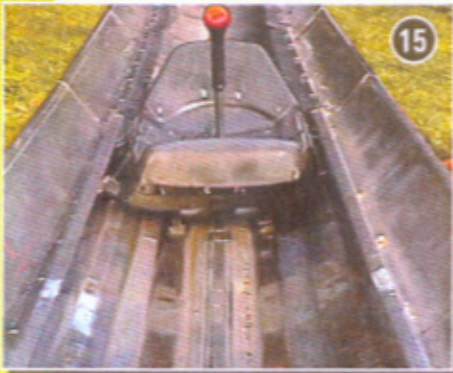
Great security with our selective braking device: only excessively rapid sleds are braked
