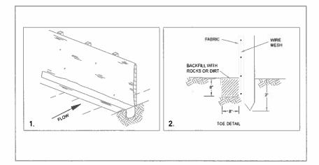
A temporary sediment barrier consisting of entrenched filter fabric stretched across and secured to supporting posts.
