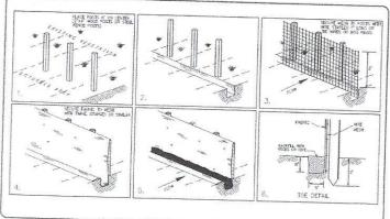
A temporary sediment barrier consisting of entrenched filter fabric stretched across and secured to supporting posts.
