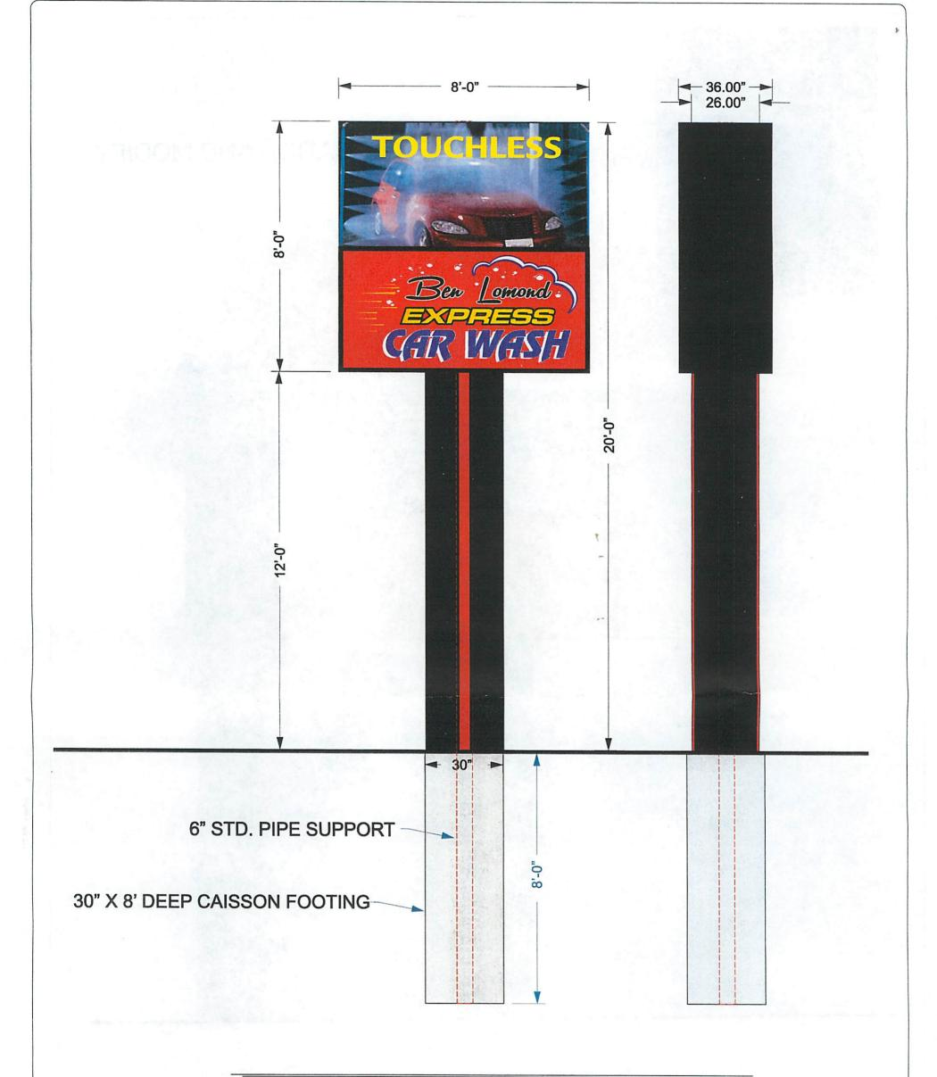
4' X 8' D/F EMC & 4' x 8' ID CABINET WITH 6" PIPE "DIRECT BURIAL" AND POLE COVER
