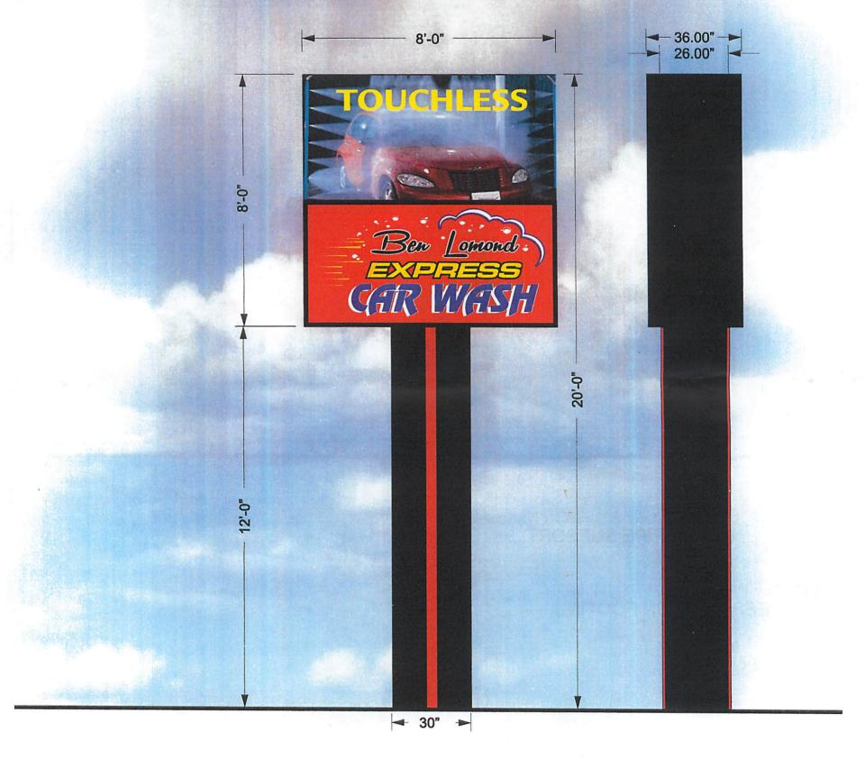
4' X 8' D/F EMC & 4' x 8' ID CABINET WITH 6" PIPE "DIRECT BURIAL" AND POLE COVER
