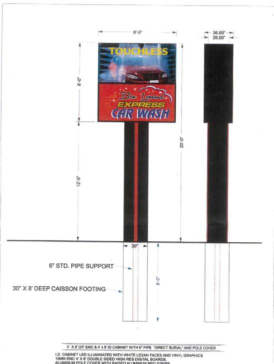
I.D. CABINET LED ILLUMINATED WITH WHITE LEXAN FACES AND VINYL GRAPHICS 10MM EMC 4" X 8" DOUBLE SIDED HIGH RES DIGITAL BOARDS. ALUMINUM POLE COVER WITH RAISED ALUMINUM RED STRIPE. INSTAL WITH 6" DIRECT BURIAL PIPE SUPPORT.
