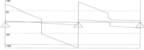
Load factor of dead load= 1 Load factor of imposed load= 1 Load width 1 (m) (by which the loads has been multiplied during calculation) Max/Min reactions of beam [kN] 79,439 205,008 25,666 4,281 22,173 -6,793
