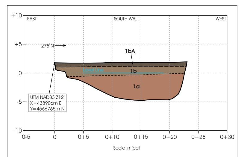
**Unit 1.** Holocene Stream Alluvium - Sequence of gravel and sand with lesser silt deposited by South Fork Ogden River comprised of a lower (1a) reddish-brown, poorly bedded, low density, gravelly sand to sandy gravel (SW/GW) with round to subround cobbles and trace boulders; and an upper (1b) reddish-brown to brown, poorly to well bedded, low density, gravelly sand to sandy gravel (SW/GW) in which the modern A-horizon soil is forming (unit 1bA).
