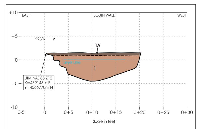
**Unit 1.** Holocene Stream Alluvium - Deposits of South Fork Ogden River comprised of brown to reddish-brown, poorly bedded to massive, low density, gravelly sand to sandy gravel (SW/GW) with round to subround cobbles and trace small boulders in which the modern A-horizon soil is forming (unit 1A); upper part slightly root penetrated.
