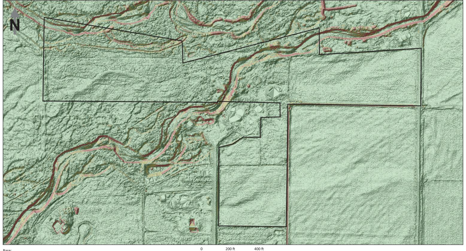
2016 LIDAR imagery available from Utah AGRC, 0.5 m resolution; slope steepness >30% shaded in red, 15-30% in yellow, and <15% in green.
