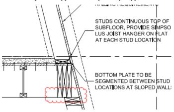
B. The supporting studs appear to be sloped. The stud capacity may be reduced. The condition also creates additional eccentricity. Please verify that this and P-detal effects have been considered.
