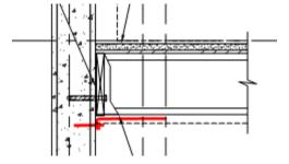
B. Diaphragms shall be provided with continuous ties or struts between diaphragm chords to distribute wall anchorage forces in to the diaphragms. Please indicate these chords on the drawing. (ASCE 7 12.11.2.2, 12.11.2.2.3)
