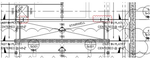
D. Please verify if wall at 1B5 is a shearwall. Walls above are shearwalls. Please verify load paths. If this is not a shearwall, the condition appears to create a vertical in-plane discontinuity irregularity. Please verify that the increase load requirements of ASCE 7 12.3.3.3, 12.3.3.4 have been satisfied. (ASCE 7 T12.3-1)
