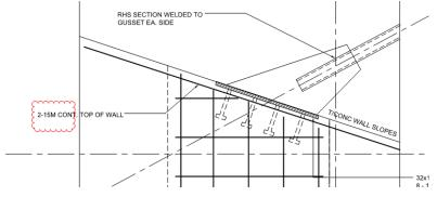
B. Detail 4, 5, 7: Please verify that diaphragm is tied to the wall. Please consider providing tension device and blocking at suitable spacing. (ASCE 7 12.11)
