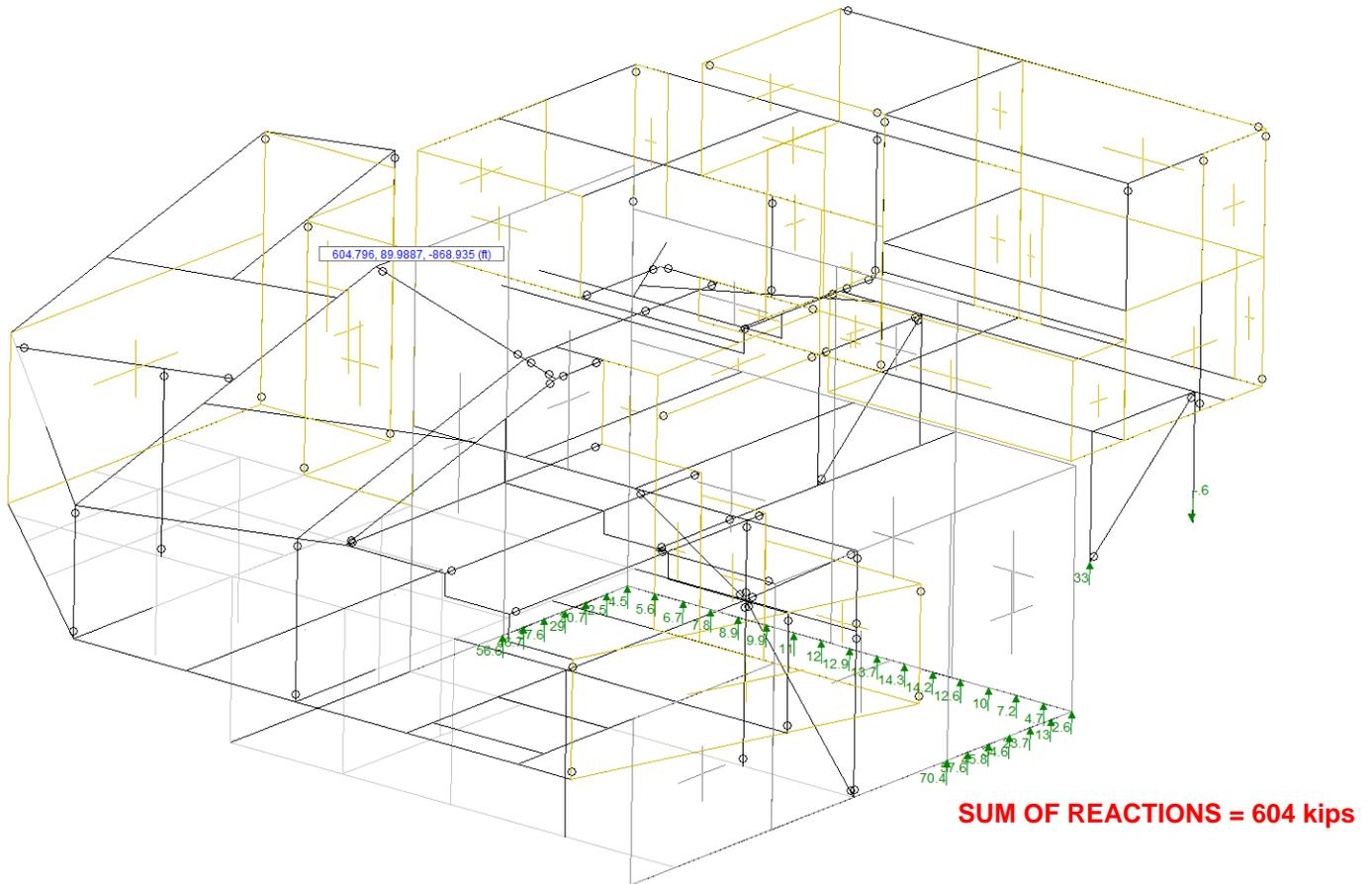
**DEAD LOAD REACTIONS (LC-2) ACTING ON THE SHALLOW FOUNDATIONS ON BEDROCK ONLY**
