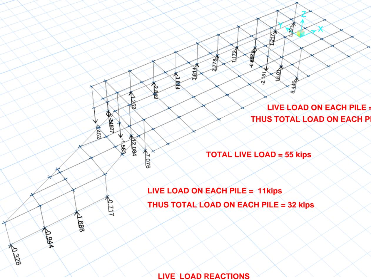
**AXIAL CAPACITY FOR 24" DIA 15' DIA PILES PER GEOTECH TABLE SHOWN IN CHAPTER 2 AND EXTRAPOLATING = 135 kips
