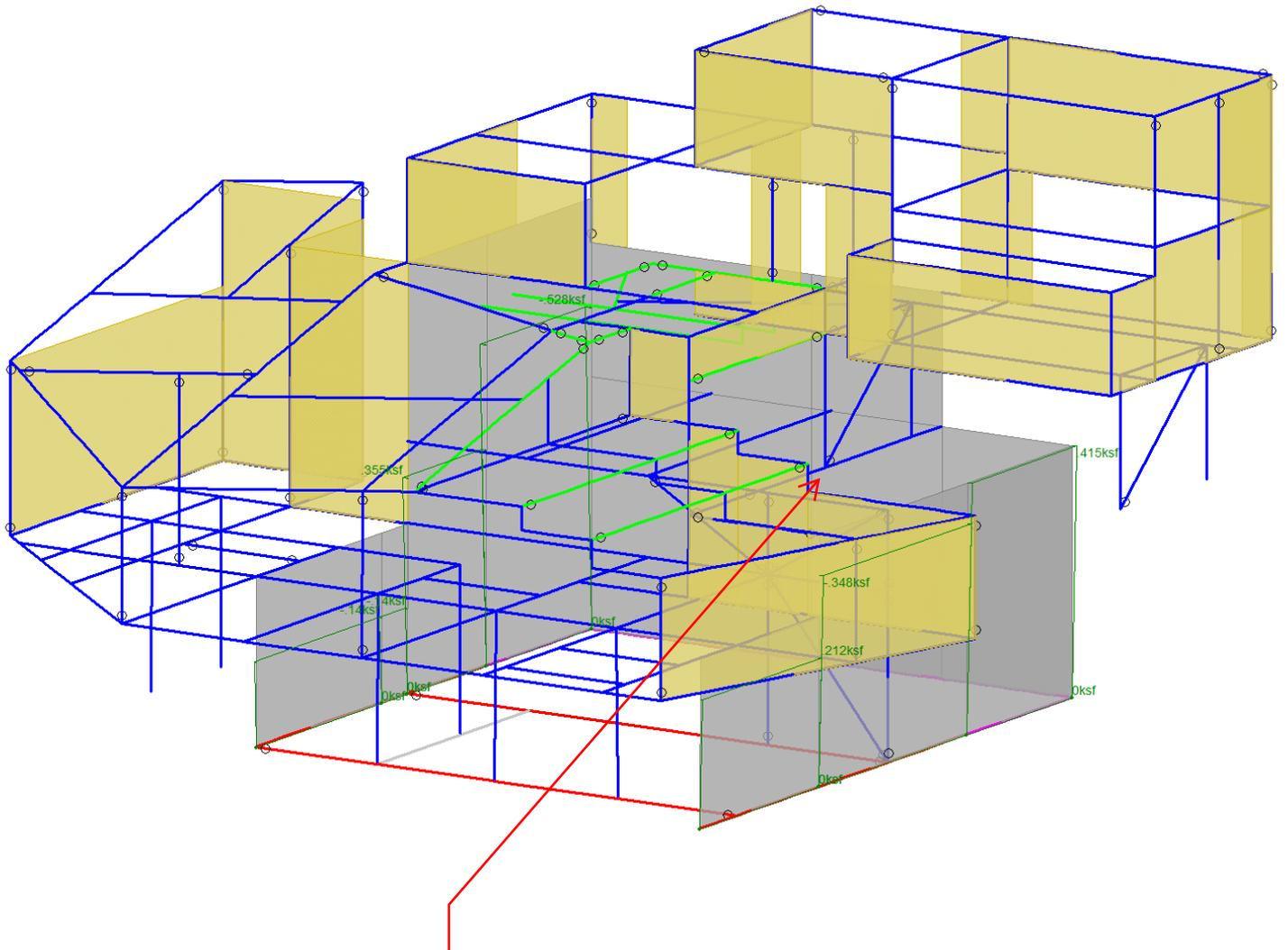
NO SEISMIC SOIL LOAD ON BACK WALL. PERMANENT SHORING WALL PROVIDED AT THE BACK INDEPENDENT FROM THE STRUCTURE. (DESIGNED BY OTHERS)
