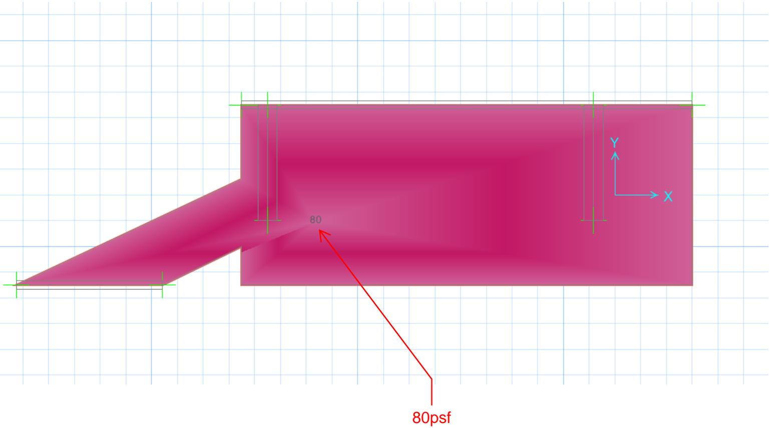
**SAFE ANALYTICAL MODEL- ASSIGNED LIVE LOAD**
