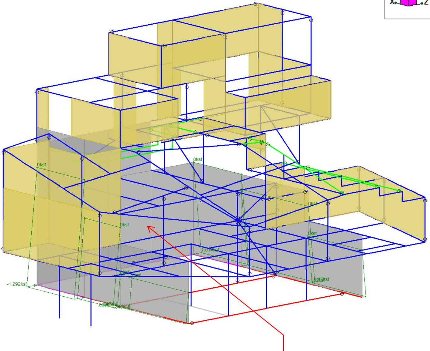
NO SEISMIC SOIL LOAD ON BACK WALL. PERMANENT SHORING WALL PROVIDED AT THE BACK INDEPENDENT FROM THE STRUCTURE. (DESIGNED BY OTHERS)
