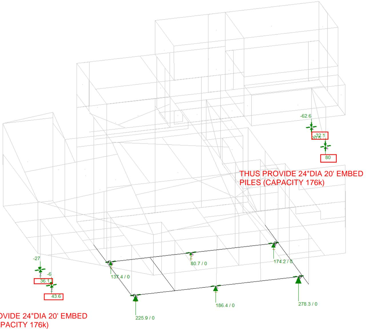
**ENVELOPE ASD AXIAL LOADS FOR PILE EMBED DEPTH DESIGN**
