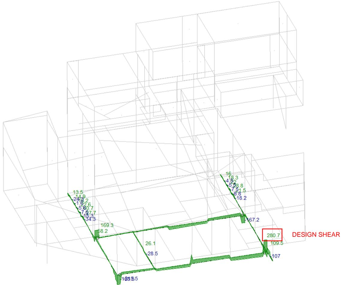
**GRADE BEAM ENVELOPE SHEAR FOR LRFD COMBINATIONS**
