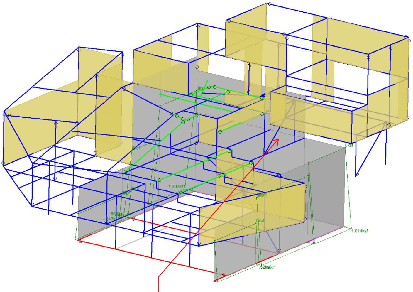
NO SEISMIC SOIL LOAD ON BACK WALL. PERMANENT SHORING WALL PROVIDED AT THE BACK INDEPENDENT FROM THE STRUCTURE. (DESIGNED BY OTHERS)
