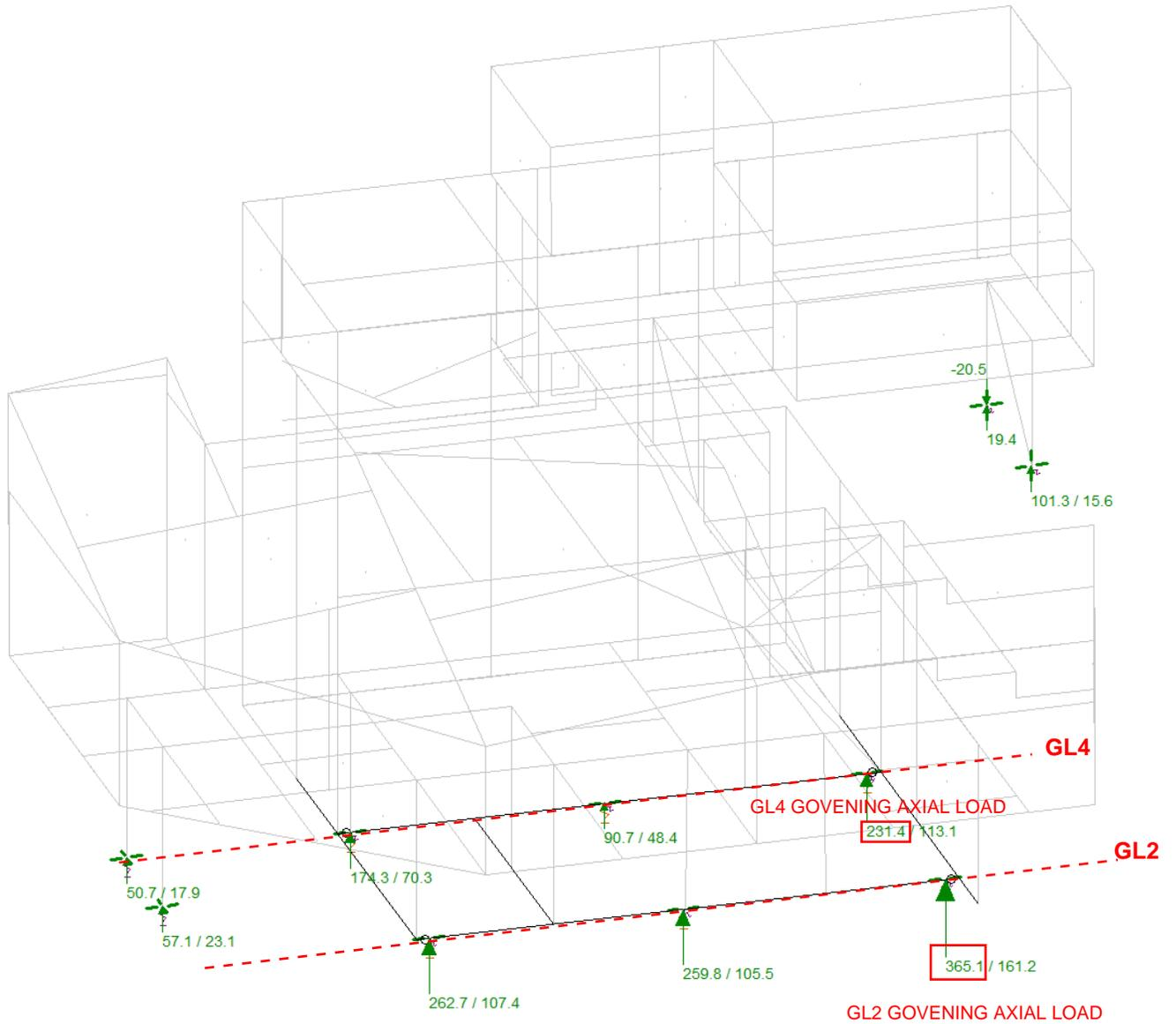
**ENVELOPE LRFD AXIAL LOADS FOR PILE STRENGTH DESIGN**
