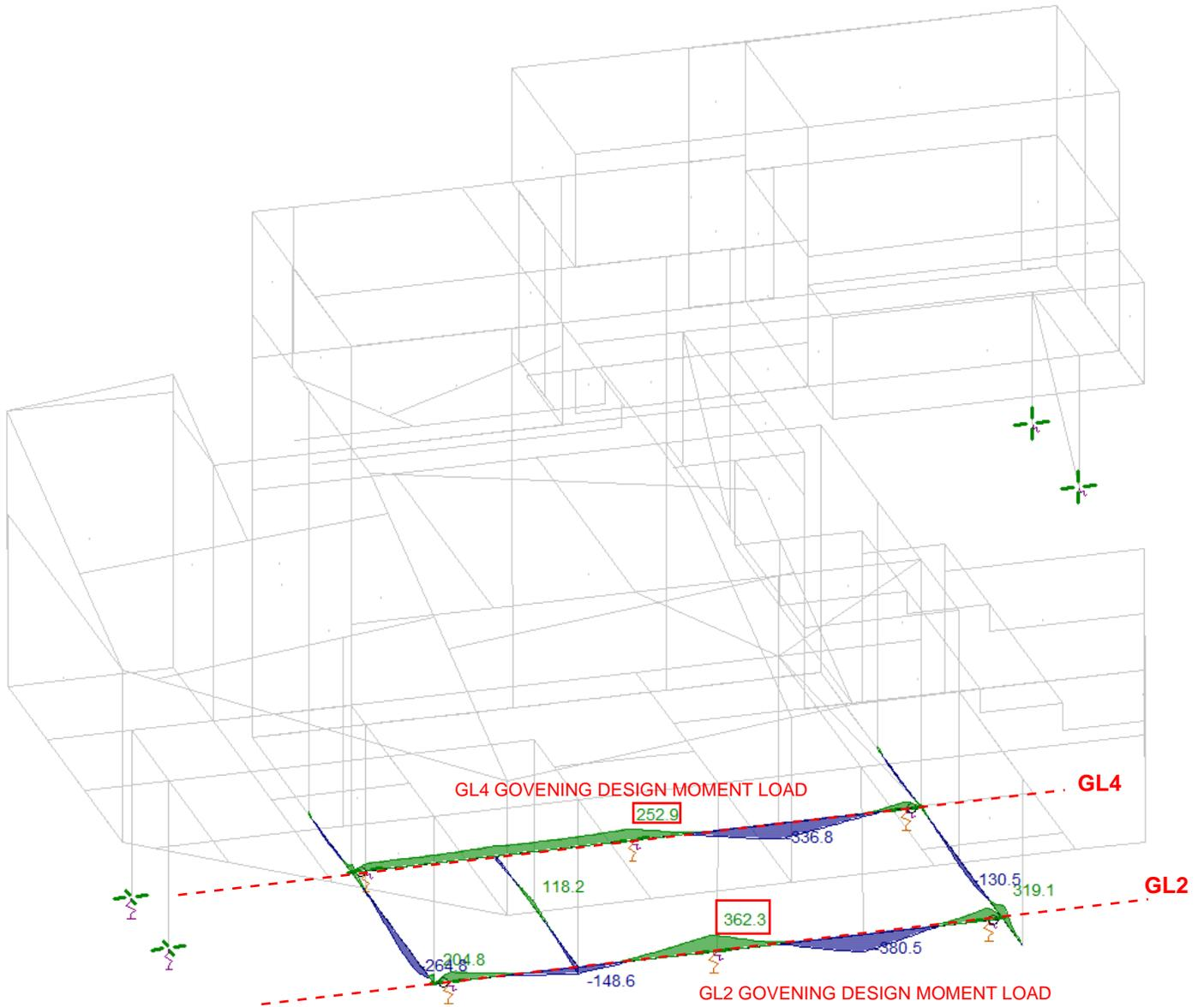
**ENVELOPE LRFD MOMENT LOADS FOR PILE STRENGTH DESIGN**
