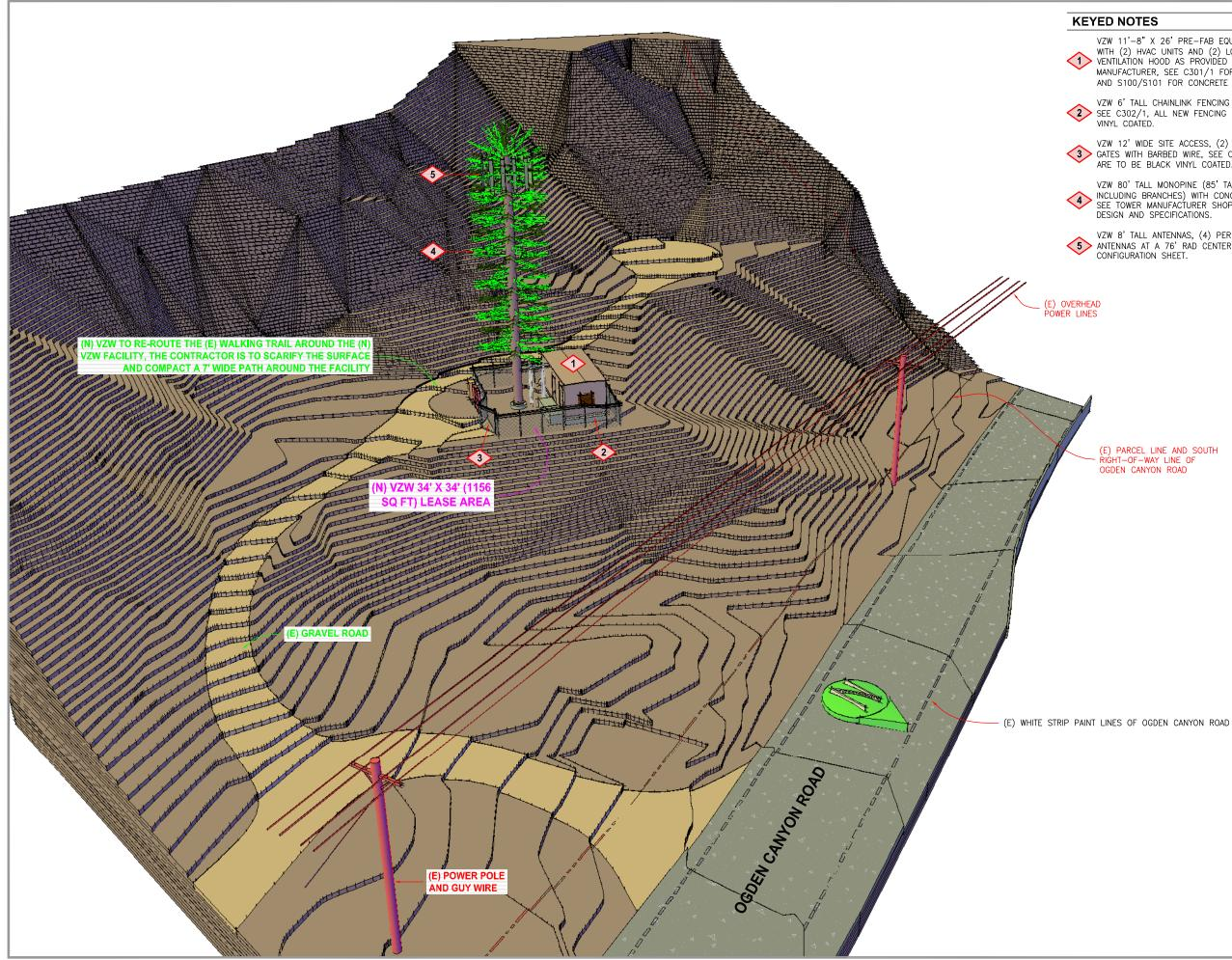
VZW 11'-8" X 26' PRE-FAB EQUIPMENT SHELTER WITH (2) HVAC UNITS AND (2) LOW PROFILE VENTILATION HOOD AS PROVIDED BY THE SHELTER MANUFACTURER, SEE C301/1 FOR EQUIPMENT LAYOUT AND S100/S101 FOR CONCRETE FOUNDATION.
