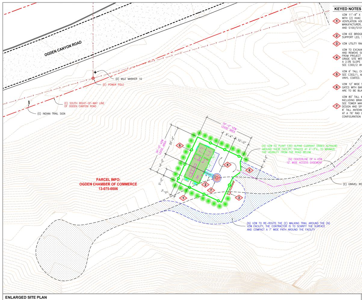
VZW 11'-8" X 26' PRE-FAB EQUIPMENT SHELTER WITH (2) HVAC UNITS AND (2) LOW PROFILE VENTILATION HOOD AS PROVIDED BY THE SHELTER MANUFACTURER, SEE C301/1 FOR EQUIPMENT LAYOUT AND S100/S101 FOR CONCRETE FOUNDATION.
