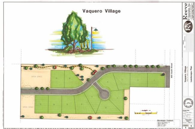
**Additional design standards and requirements:** A large irrigation ditch crosses along the north boundary of the subdivision. Irrigation ditches or canals which carry five second feet or more of water is required to install a solid board, chain link, or other non-climbable fence not less than five feet in height. Therefore, if required by the volume of water, the applicant will have to install a non-climbable fence of not less than five feet along this irrigation ditch.
