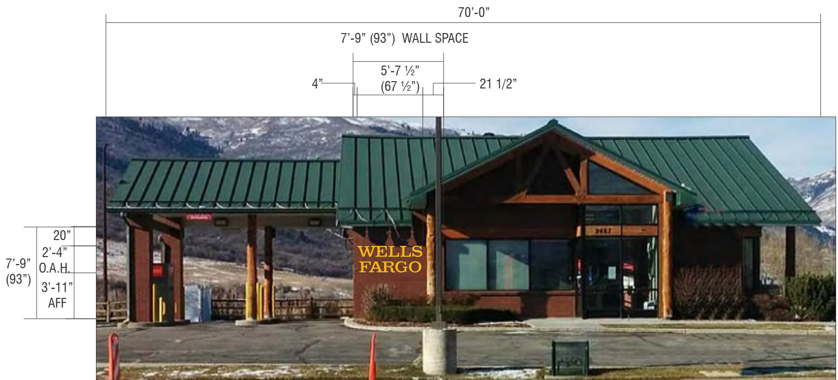
NE03 PROPOSED CPL-12-ST-GNL SIGN ELEVATION SCALE: 1/8" = 1'-0"
