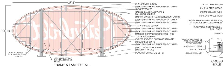
FRAME & LAMP DETAIL SCALE: 3/16" = 1'-0"
