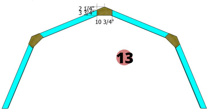
Use 1/2" plywood for the gussets. Mark the cut lines on the plywood and get the job done with a circular saw. Lay the gussets over the joints, as shown in the diagram.
