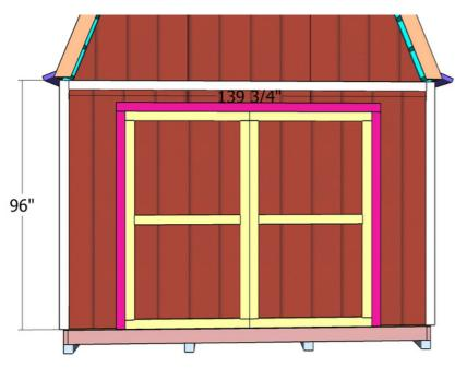
Fit the 1x4 trims to the front and back of the storage shed.
