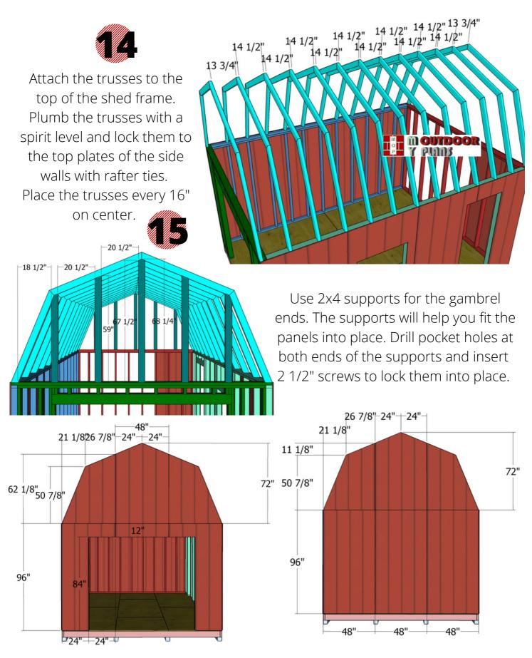
Attach the 5/8" T1-11 siding sheets to the front and back of the shed. Align the edges flush and use 6d nails, every 8" along the framing, to lock them into place. Use a saw to make the cuts around the double door opening, as well as to the gambrel end panels.
