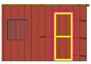
Fit the door to the opening, align the edges and lock it to the jambs with hinges. Install a latch so you can lock the door. Alternatively, you can install a pre-hung door.
