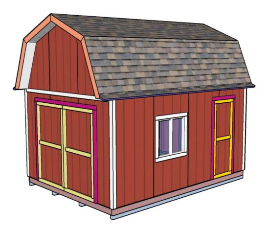
Last but not least, you need to take care of the finishing touches. Fill the holes with wood putty and smooth the surface with sandpaper. Apply a few coats of paint to protect the exterior of the shed from the elements.
