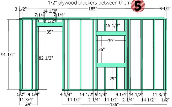
Next, assemble the other side wall for the shed. Use the same techniques described above. Notice the window and the door openings, with the double studs and the double 2x6 headers. You can adjust the location and the size of the openings to suit your needs.
