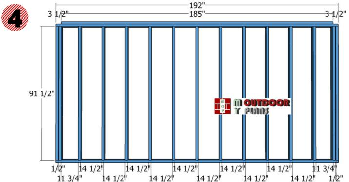
Next, assemble the side wall frame. Cut all the components from 2x4 lumber. Lay the components on the shed floor and attach the studs to the plates, every 16" on center. Use 3 1/2" nails or screws, through the plates into the studs. If you use screws, drill pilot holes. Notice the double studs placed at both ends, with
