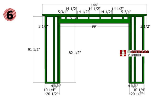
Next, build the front wall for the garden shed. As you can see in the diagram, I have designed it with a 8 ft opening, so you can install double doors and have easy access inside the shed with larger objects. Notice the 2x6 double header. Measure the diagonals of the wall frame and make sure they are equal. In addition, check if the corners are square when installing the studs.
