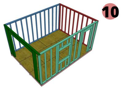
Next, attach the front and back wall frames to the floor of the shed. Make sure the edges are flush and then insert the 3 1/2" screws through the plates into the shed floor.
