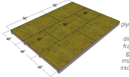
Use 3/4" pressure treated plywood for the floor of the shed. cut the sheets at the right dimensions and lay them to the frame. Align the edges, leave no gaps between the sheets and insert 1 5/8" screws to lock them into place. Insert the screws every 8" along the framing.
