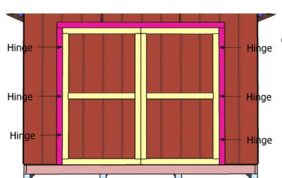
Fit the double doors to the opening and use hinges to secure them to the jambs. Install a latch to keep the doors locked.
