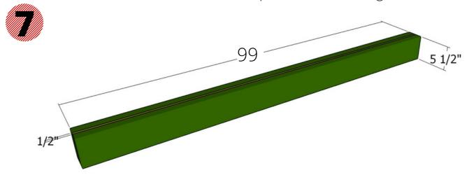
Make sure you build the header separately, by gluing 2x6s to a piece of 1/2" plywood. Add glue to the joinsts and insert 2 1/2" nails from both sides.
