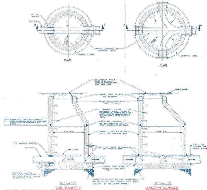
8 TYPICAL SANITARY SEWER MANHOLE
