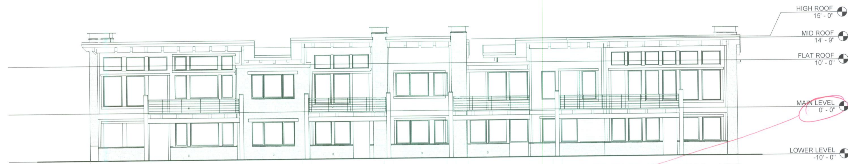
SOUTH ELEVATION BUILDINGS 1-4 100'-00" = 5218.70 BUILDINGS 5-8 100'-00" = 5220.00
