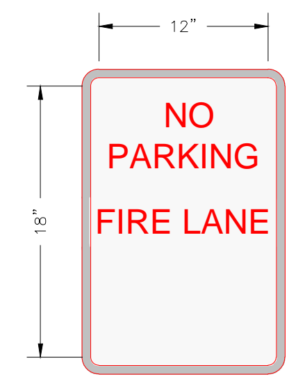
4 FIRE LANE SIGN DETAIL Scale: NTS
