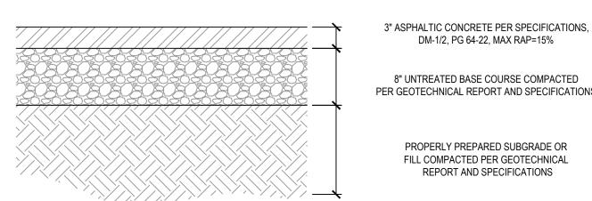
8" UNTREATED BASE COURSE COMPACTED PER GEOTECHNICAL REPORT AND SPECIFICATIONS PROPERLY PREPARED SUBGRADE OR FILL COMPACTED PER GEOTECHNICAL REPORT AND SPECIFICATIONS
