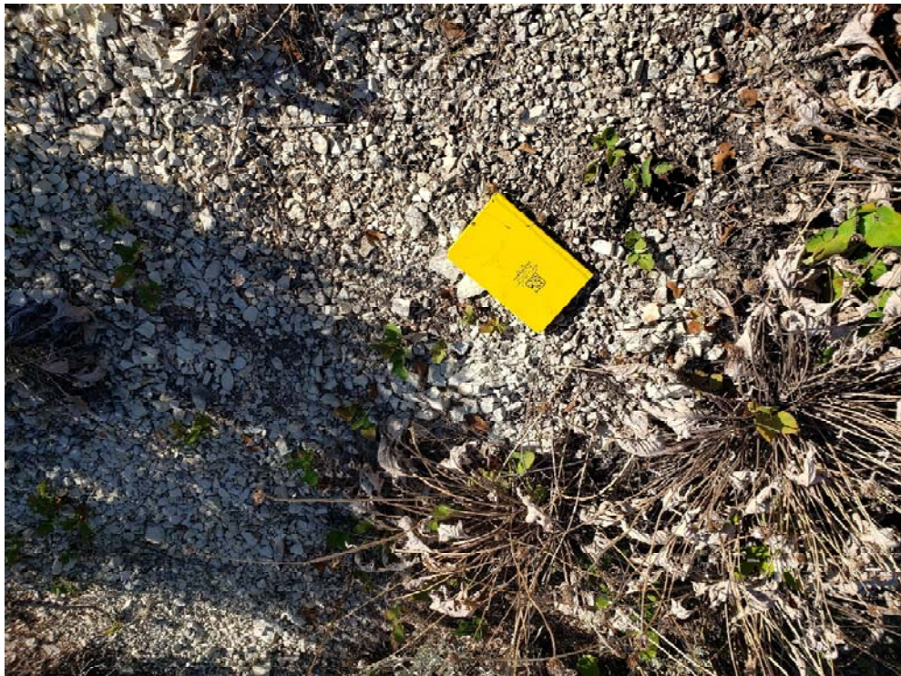
Photo 6. Typical weathered Norwood Formation sandstone bedrock at surface
