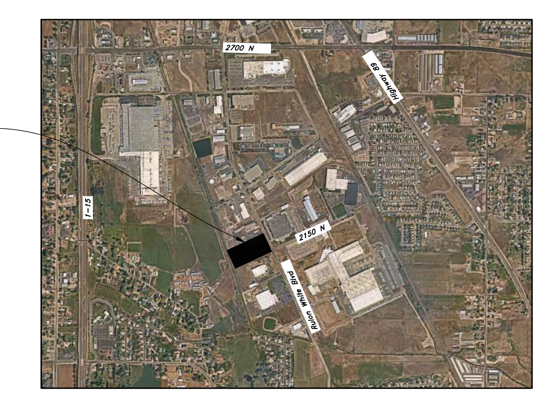
VICINITY MAP Not to Scale Benchmark #9005 Brass Cap Monument Of Intersection Of 2150 North Street and Rulon White Blvd Elev = 4283.62'
