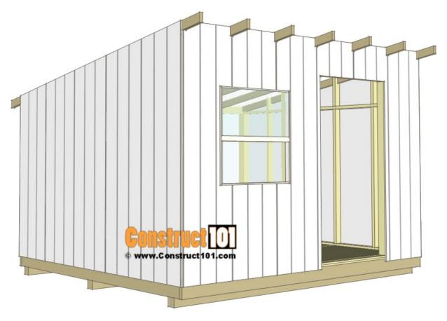
Measure and cut the t1-11 exterior siding to size, notch front and back siding around rafters. Install siding using 2" finishing nails.
