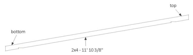
Cut seven 2×4's to 11' 10 3/8" for the rafters. Cut the ends of the rafters as shown on illustration below.
