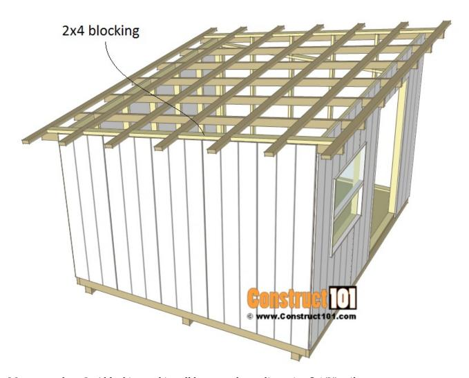
Measure and cut 2×4 blocking and install between the purlins using 3 1/2" nails.
