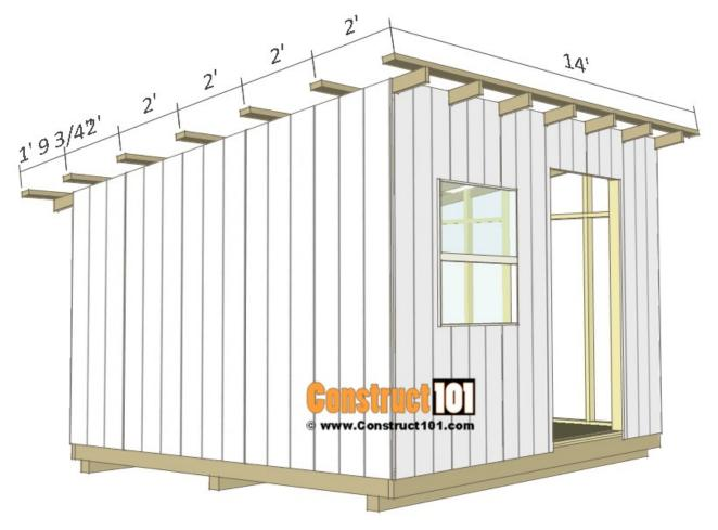
Cut seven  $2\times4$ 's to 14' long for the purlins. Install purlins as shown on illustration above using  $3\ 1/2''$  nails.
