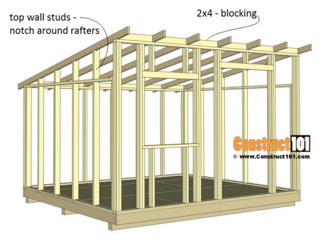
Measure and cut the top wall studs for the side walls to size, notch around rafters and install using 3 1/2" nails.
