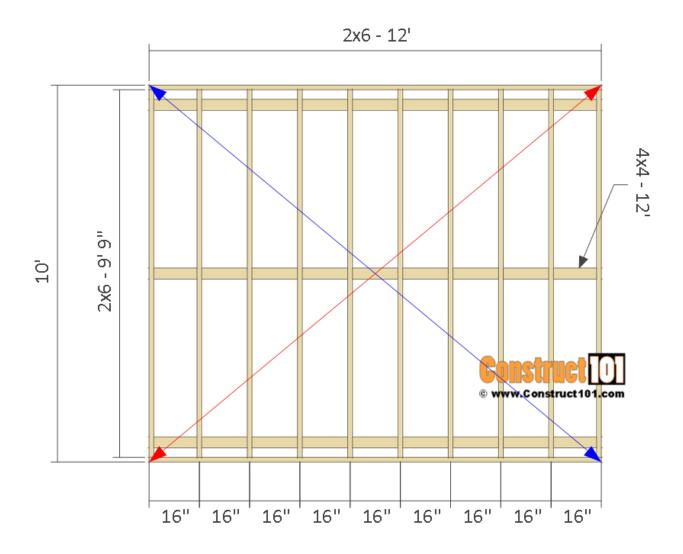
Cut two  $2\times6$ 's to 12' long for the floor band. Cut ten  $2\times6$ 's to 9' 9'' for the floor joist. Cut three  $4\times4$ 's to 12' long for the skids.
