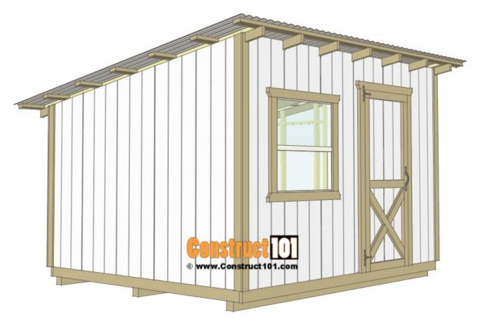
Measure and cut  $1\times4$ 's to size for the corner and window trim. Install the  $1\times4$  trim using 2'' finishing nails.
