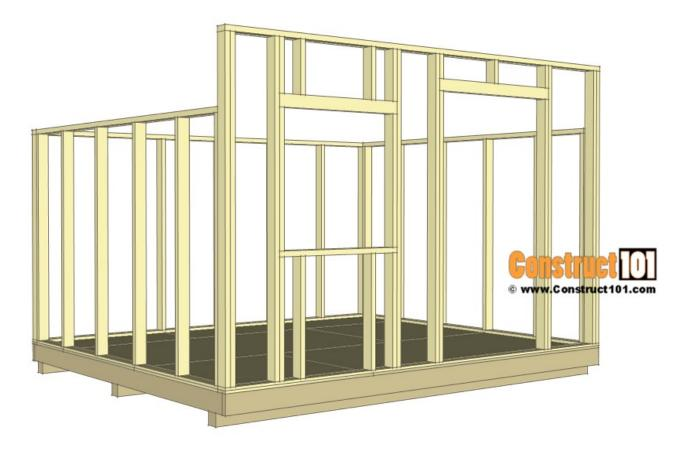
Secure the wall frames using 3 1/2" nails.
