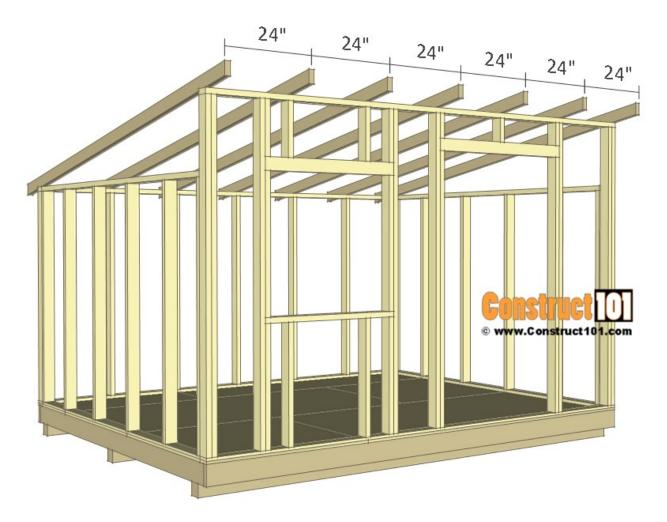
Rafters are spaced out 24" O.C., install using 3 1/2" nails.
