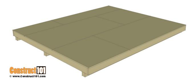
Measure and cut to size the 3/4" tongue and groove floor deck.
