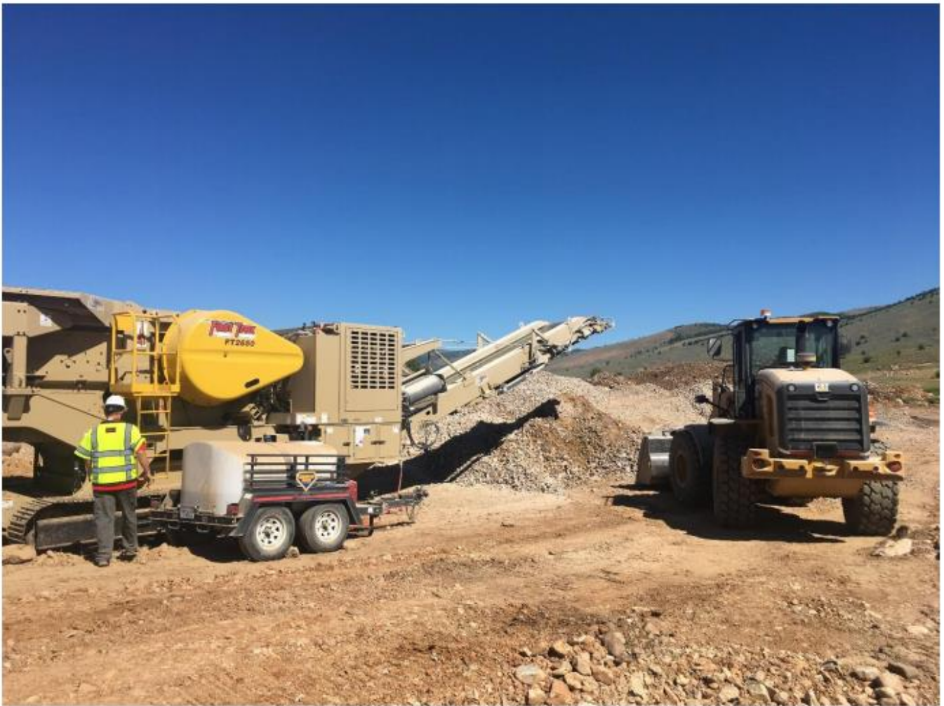
Example photo of the type of crusher proposed to repurpose the boulders onsite into structural fill
