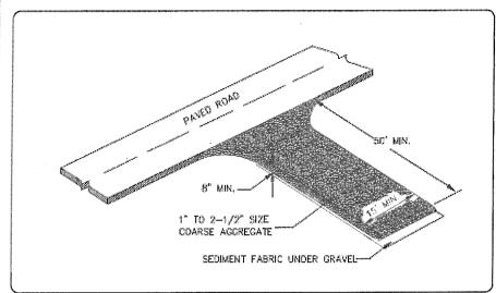
A stabilized pad of crushed stone located where construction traffic enters or leaves the site from or to paved surface.
