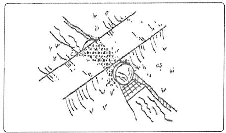
A temporary access stream crossing is a temporary culvert, ford or bridge placed across a waterway to provide access for construction purposes for a period of less than one year. Temporary access crossings are not intended to be used to maintain traffic for the general public.
