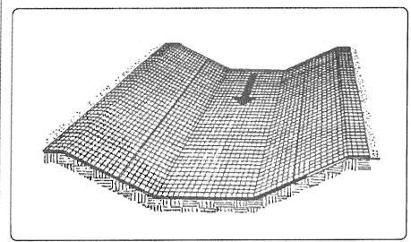
Erosion control blankets are used in place of mulch on areas of high velocity runoff and/or steep grade, to aid in controlling erosion on critical areas by protecting young vegetation.
