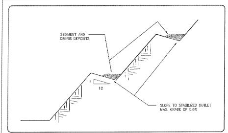
Slope construction with benches spaced at regular intervals perpendicular to the slope which intercept and collect sheet flow and direct it to a stable outfall point.
