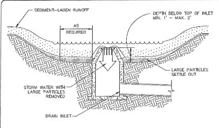
An area excavated around a storm drain inlet to impound water below the inlet.
