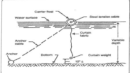
A flotation silt curtain is a silt barrier for use within a lake or pond. The flotation silt curtain consists of a filter fabric curtain weighted at the bottom and attached to a flotation device at the top. This structure is used to isolate an active construction area within a lake or pond to prevent silt-laden water from migrating out of the construction zone.
