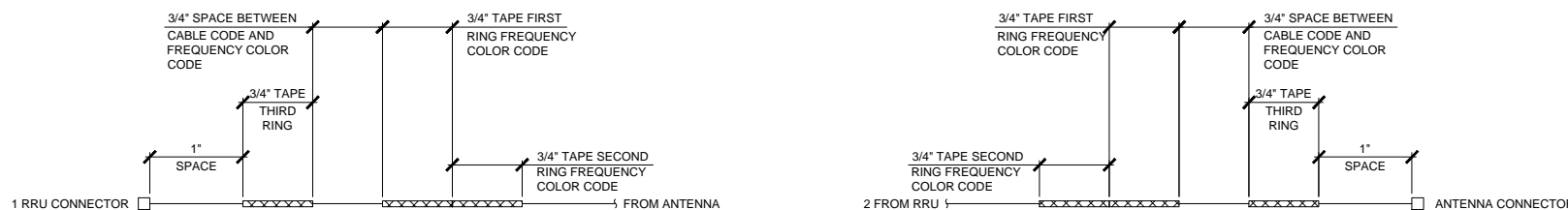
JUMPER CABLE CONNECTION AT RRU AND ANTENNA
