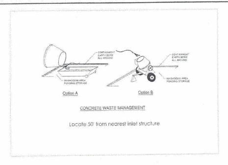
Prevent or reduce the discharge of pollutants to storm water from concrete waste by conducting washout off-site, performing on-site washout in a designated area, and training employees and subcontractors.
