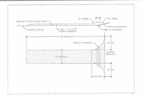
A stabilized pad of crushed stone located where construction traffic enters or leaves the site from or to paved surface.
