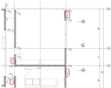
There is an open-ended diaphragm at the garage. The forces in the shear walls surrounding the garage have been increased as required. The shear wall and holdown callouts are correct.
