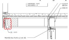
The connection is correct. This is not a cantilever. The double rim is supported by the steel beams.
