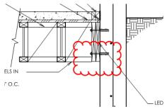
Straps have been added to eliminate the potential cross grain bending in the ledgers. See updated drawings.
