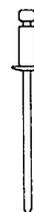
Pop Rivet Used For: -Trim Lap -Downspout to Gutter -Outside Corner Box -Downspout Strap
