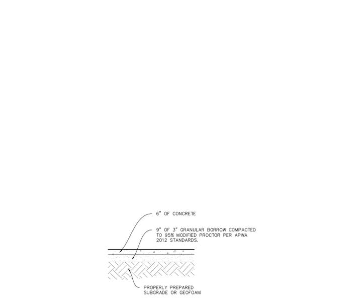
**CONCRETE DRIVEWAY PAVEMENT SECTION** NTS
