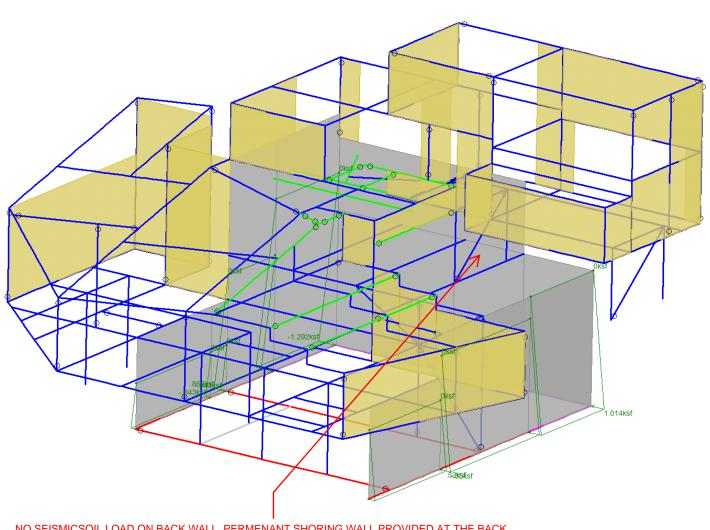
NO SEISMICSOIL LOAD ON BACK WALL. PERMENANT SHORING WALL PROVIDED AT THE BACK INDEPENDENT FROM THE STRUCTURE. (DESIGNED BY OTHERS)
