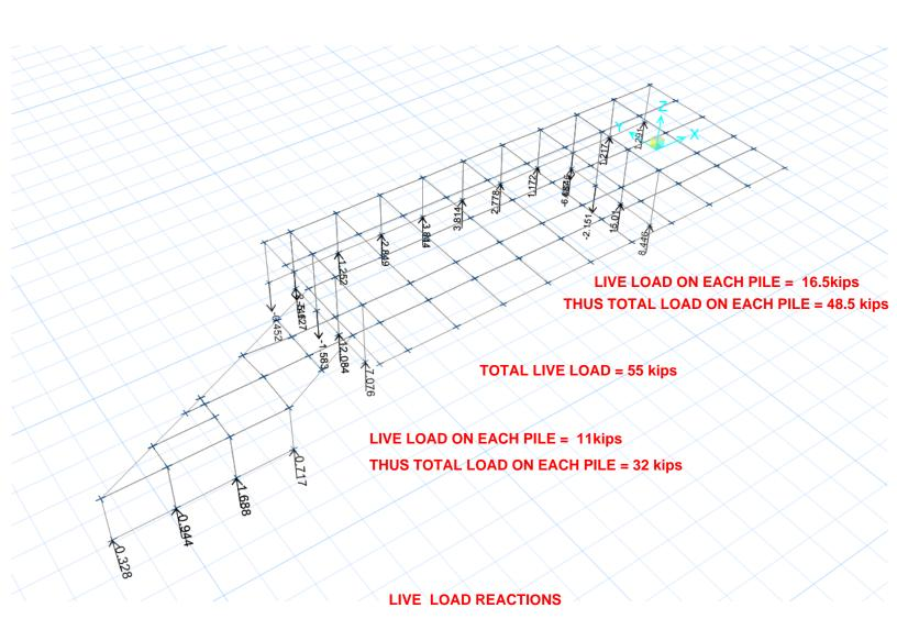
AXIAL CAPAPCITY FOR 24" DIA 15' DIA PILES PER GEOTECH TABLE SHOWN IN CHAPTER 2 AND EXTRAPOLATING = 135 kips THUS 15' EMBED IN BEDROCK OKAY FOR AXIAL LOADS
