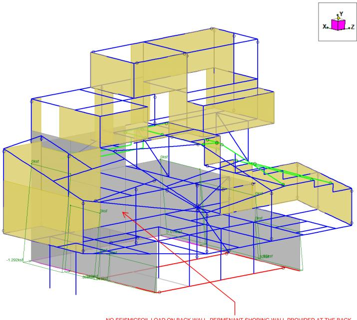
NO SEISMICSOIL LOAD ON BACK WALL. PERMENANT SHORING WALL PROVIDED AT THE BACK INDEPENDENT FROM THE STRUCTURE. (DESIGNED BY OTHERS)
