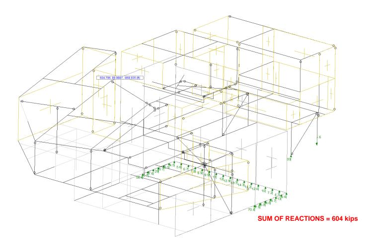
DEAD LOAD REACTIONS (LC-2) ACTING ON THE SHALLOW FOUNDATIONS ON BEDROCK ONLY
