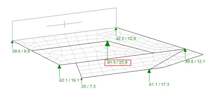
THUS PROVIDE PILES 24" DIA 15' EMBED IN BEDROCK. AXIAL CAPACITY FOR 15' EMBED IN BEDROCK PER GEOTECH REPORT = 135 kips. THUS OKAY.
