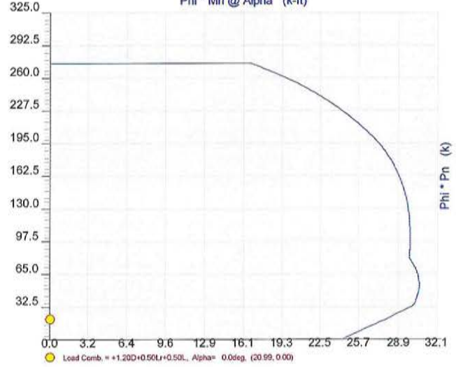
Concrete Column P-M Interaction Diagram
