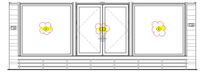
B. The window in the master bedroom does not meet the requirements for emergency escape and egress openings, as required by IRC R310.1.
