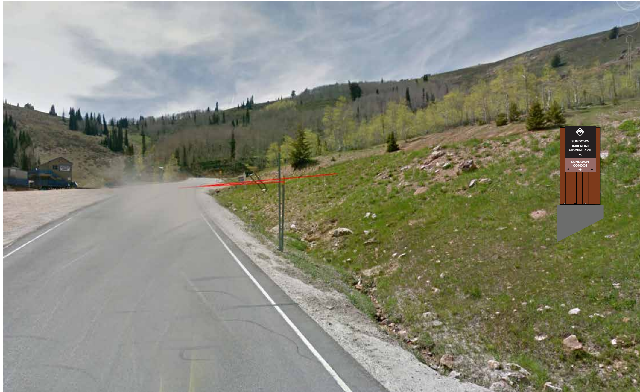
ST ~ 2.1 / ELEVATION VIEW / 50'-0" SETBACK FROM CENTERLINE ON ST ROUTE 158. This is an approximate scale & position, exact location will be determined and identified to UDOT & Weber County Planning Department prior to fabrication and installation.
