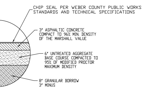
SUBGRADE PREPARATION SHOULD INCLUDE REWORKING AND COMPACTING THE UPPERMOST 12-INCHES OF NATIVE SOILS TO A MINIMUM OF 95 PERCENT OF THE MDD AS DETERMINED BY ASTM D-1557.
