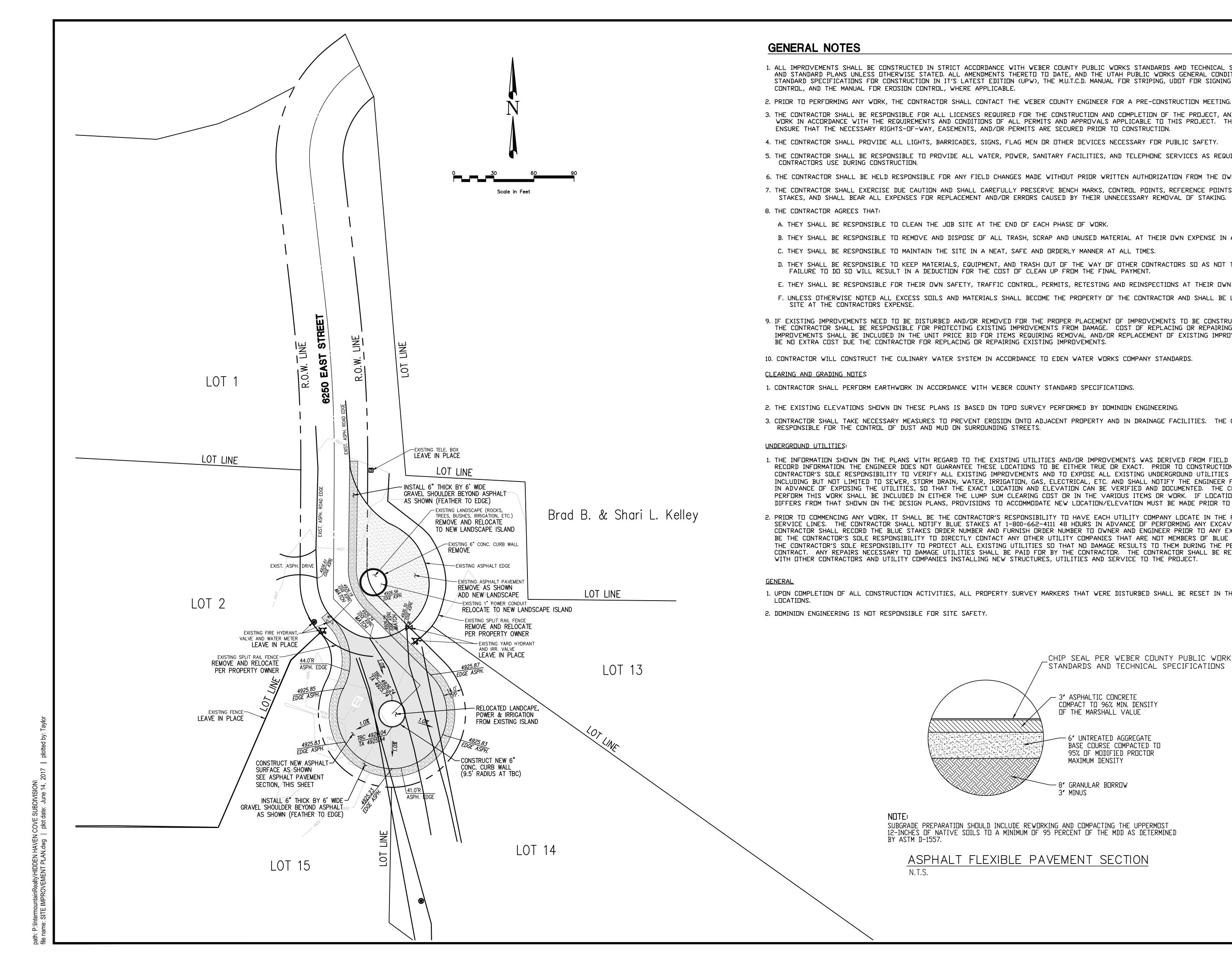
1. ALL IMPROVEMENTS SHALL BE CONSTRUCTED IN STRICT ACCORDANCE WITH WEBER COUNTY PUBLIC WORKS STANDARDS AMD TECHNICAL SPECS. APWA SPECIFICATIONS AND STANDARD PLANS UNLESS OTHERWISE STATED. ALL AMENDMENTS THERETO TO DATE, AND THE UTAH PUBLIC WORKS GENERAL CONDITIONS AND STANDARD SPECIFICATIONS FOR CONSTRUCTION IN IT'S LATEST EDITION (UPW), THE M.U.T.C.D. MANUAL FOR STRIPING, UDDT FOR SIGNING AND TRAFFIC
