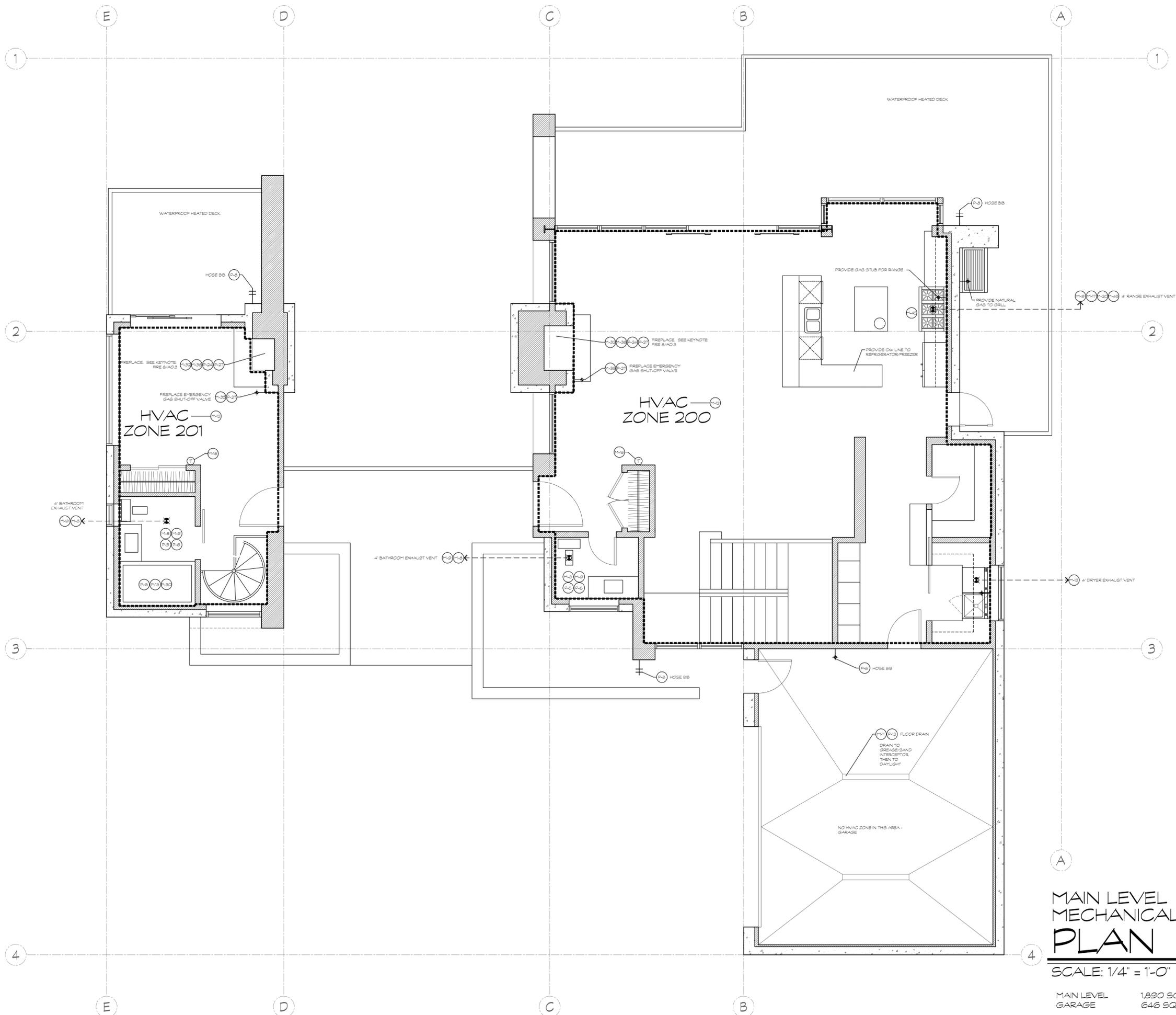
MECHANICAL/PLUMBING LAYOUTS ARE SHOWN IN SCHEMATIC. THE CONTRACTOR IS RESPONSIBLE TO COORDINATE THE LAYOUT AND INSTALLATION OF ALL RELATED ITEMS WITH EXISTING CONDITIONS AND RELATED TRADES.
