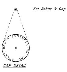
A 5/8"ø rebar 24" long with plastic cap (see detail above) was set at all property corners as shown.
