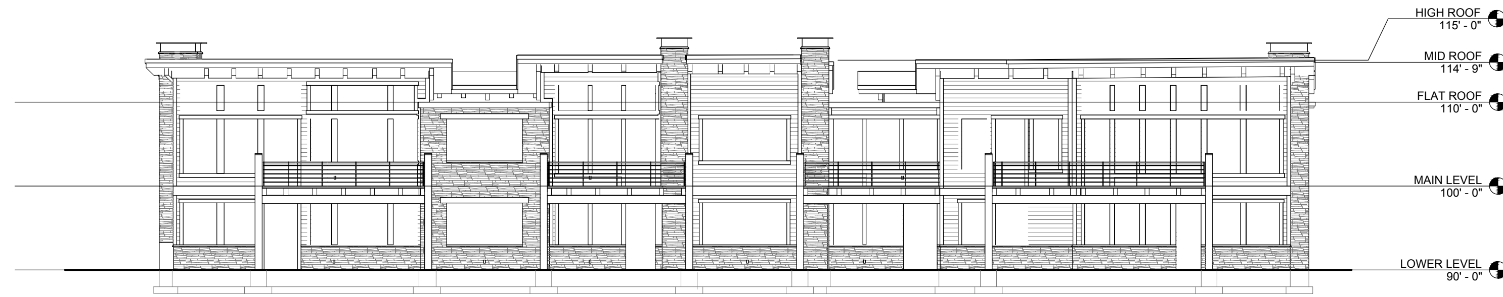
SOUTH ELEVATION BUILDINGS 301-304 100'-00" = 5242.50 BUILDINGS 401-404 100'-00" = 5245.00
