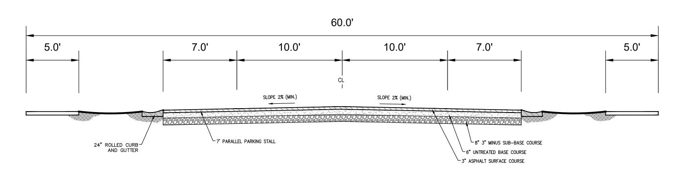
NOTE: ALL DEPTH STANDARDS ARE MINIMUM AND MORE CAN BE REQUIRED BASED ON GEOTECHNICAL REPORT
